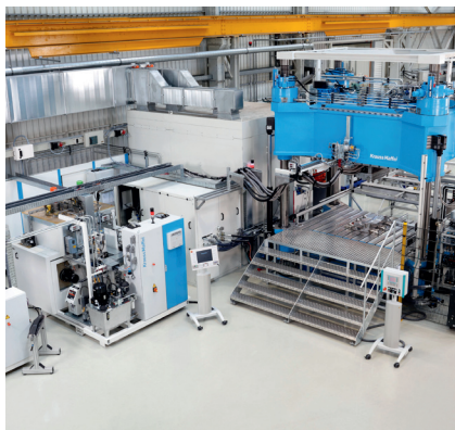
A laboratory production facility for the high pressure RTM process, featuring a Krauss Maffei dosing unit, high pressure RTM mixing head and mould carrier.
