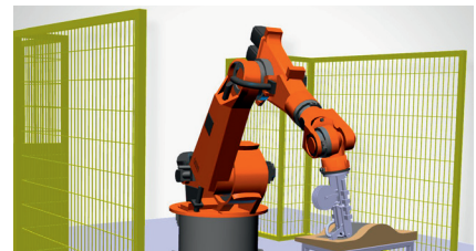
SWMS' TapeStation is an independent programming and simulation software which has been developed for the automated lay-up of reinforced tows and tapes.
